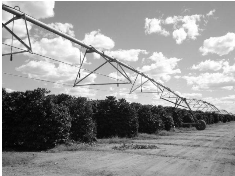
Figure 2. View of a central pivot system equipped with Low Energy Precision Application (LEPA) sprinklers, in a commercial coffee plantation. Barreiras, Bahia State, Brazil.
